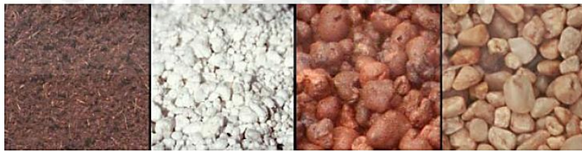
Gambar 2–21 Media tumbuh hidroponik (kiri-kanan); coconut coir, agricultural grade perlite, expanded clay pellets, and common pea gravel.
