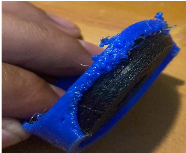
Gambar 4.31 Hasil 3D print overhead
